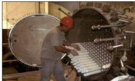
Figure 2-7: A typical cartridge filter arrangement
