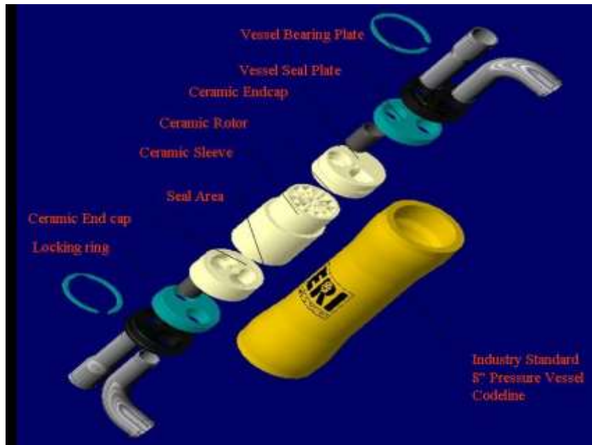
Figure 2-8: Energy Recover Inc. pressure exchanger
